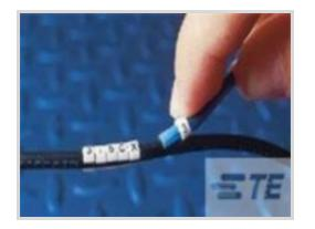
Marker Style: Snap-On Marker Size: STD 17 Compatible Cable Diameter Range: 8.5 – 11.5 mm [ .335 – .452 in ] Marker Cut: Straight Printed Marking: H All STD Snap-On Markers (966)
